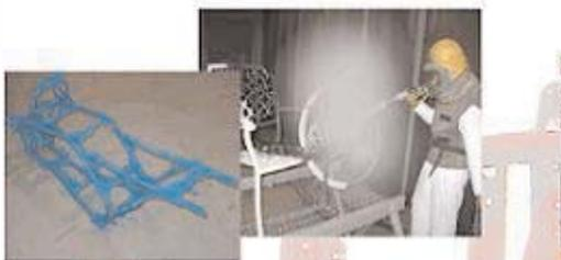
**Our 10 ft x 10 ft x 25 ft media blasting booth allows for large items such as panels and frames to be properly prepared for powder coating.**
